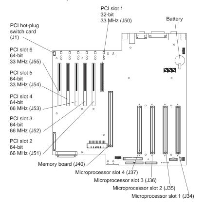
**System board cable connectors:** The following illustration shows the location of the cable connectors on the system board.
